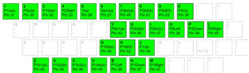
Figure 86: Key map used for browser control of the Arduino to JAMMA connection.
