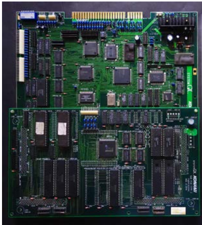
(a) JAMMA compatible PCB with the 56-pin connector shown at the top.
