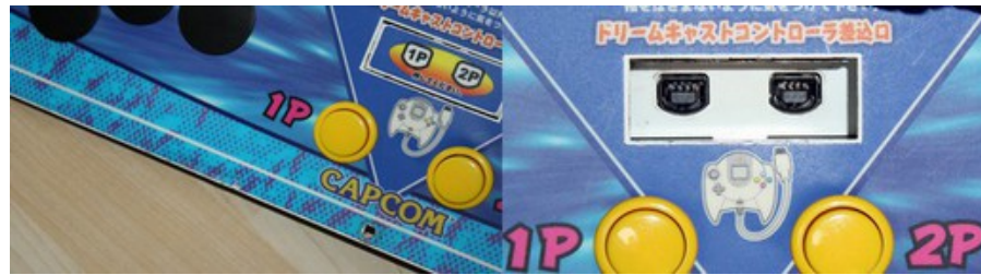
Figure 27: Sega Dreamcast enabled control panel.
