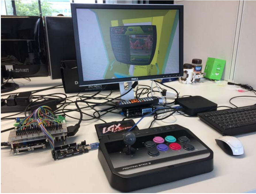
Figure 88: The VR SuperGun prototype set up in desktop mode using a flat monoscopic 3D display.
